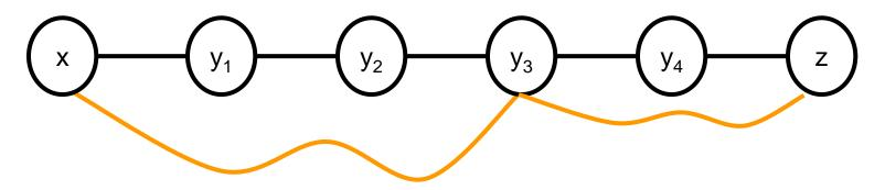
A minimum cost path from x to z. One of its subpaths is a path from x to the intermediate node  $y_3$ .
