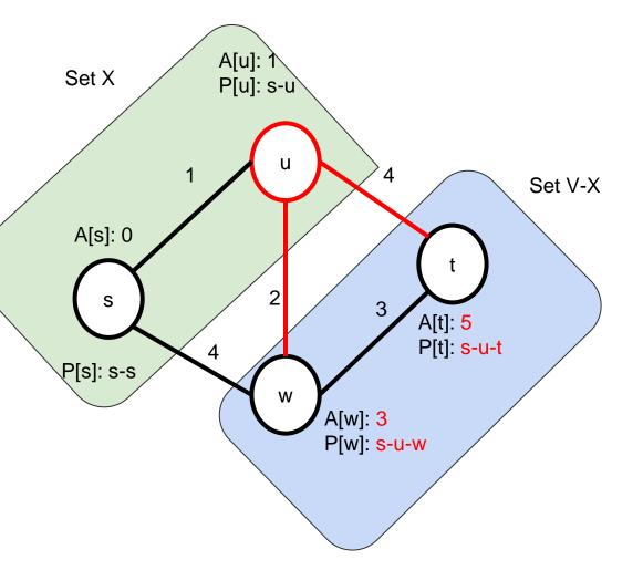
• We check if we can update the DGS using A[u] + cost(u,t) and A[u]+cost(u,w)
