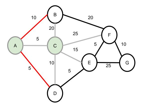
Update DGS for every node v adjacent to A: cost of path(C-A) + cost of edge(A, v) Select the node with min DGS and add it to Processed
