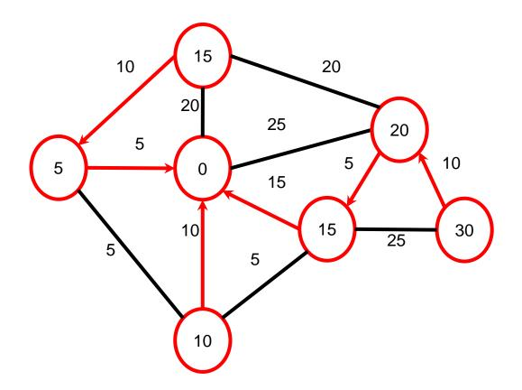
Of course, instead of storing the actual min path for each node, we could just store the cost of the path and the link to the parent node when we update DGS, and we will be able to find the shortest path from any node to C
