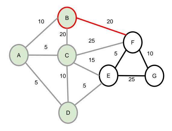
Update DGS for all unprocessed nodes v adjacent to B: cost of min path(C-B) + cost (B,v) Select the node with min DGS and add it to known min-cost paths
